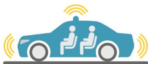
**Level 3** - Conditional automation. The system can perform the driving functions in certain scenarios. The system notifies the driver when its limits are reached. The driver does not need to monitor the system but must assume control within a certain time frame upon the system’s request.
