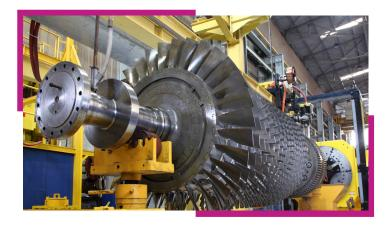
Steam turbines rotate from pressurized steam. Unlike gas turbines, steam is generated outside of the turbine, usually in a boiler that can be fueled by burning coal or gas, or absorb heat from the decay of radioactive fuel.
